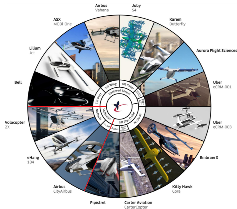
Figure 2.27: Wheel of concepts. Right side outside the red line are fixed-wing configuration [47]
