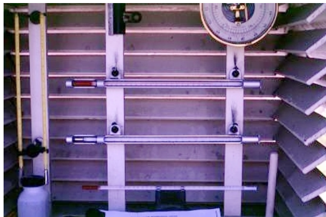
Figure 8-2: Thermometers found inside the instrument shelter are mounted approximate 1.5 meters above the ground surface. The top thermometer contains alcohol and is used to determine daily minimum temperatures. The lower thermometer uses mercury to determine the daily maximum temperature.
