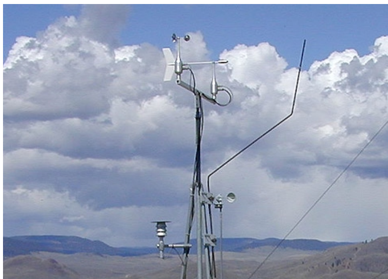
Figure 14-2: Meteorological instruments used to measure wind speed and direction.
