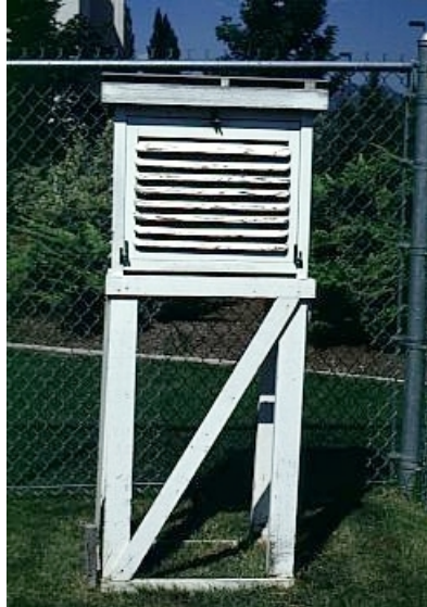
Figure 8-1: Well ventilated instrument shelters are used to protect thermometers from precipitation, direct sun, and other physical elements. Construction standardisation of these shelters, by international agreement, guarantees that measurements are comparable in any of the over 15,000 weather stations found worldwide.
